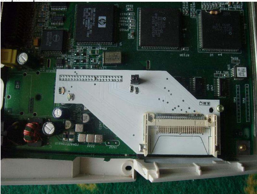
Here are 2 examples of the PCMCIA sockets I have on my A1200's . The shallow one below is not suitable for using a screw to secure the adapter in place and a dab of superglue or hot glue would be preferred to secure the adapter in place. The adapter does a good job of being held in place just by the IDE connection alone but extra securing is always good to reduce stress on the pins.
