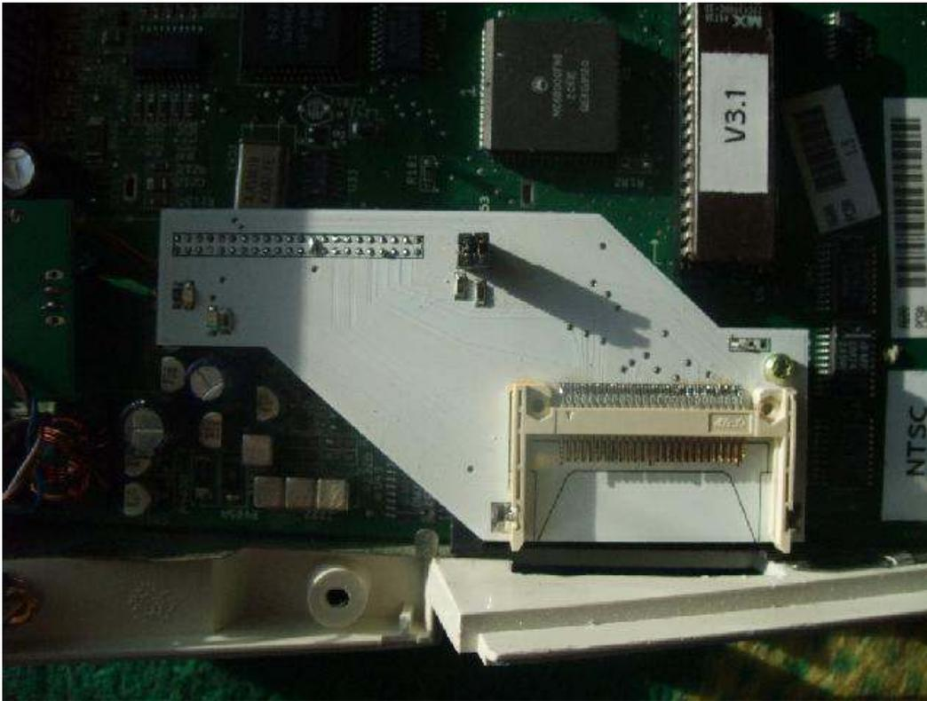
Below is the adapter installed in the A1200, note the different location of the securing screw. I have 2 different types of PCMCIA sockets in my A1200 collection, one type works fine, the other not so good (pictures further down. If you have the shallow type slot then you should use a little super glue to secure the adapter in place.
