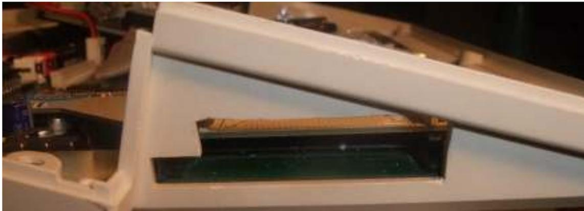
A dremel is the tool of choice to cut out the plastic. Cut on the inside of the lines to allow for minor corrections. I used a coarse file to flatten out the bumps a bit.
